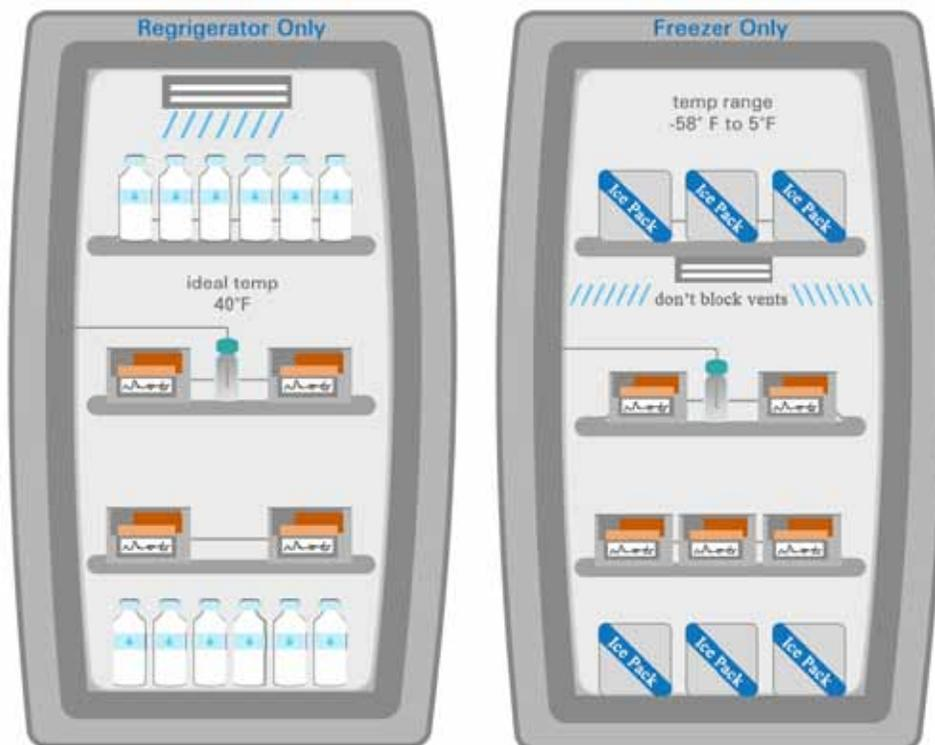
Place water bottles on the top shelf, floor, and in door racks of refrigerator.
