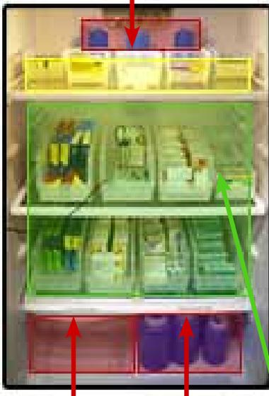
No storage in crisper drawers: thermally isolated + floor level runs cold. Remove drawers, fill space with water bottles.
