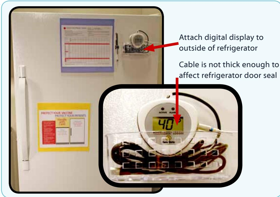
Attach digital display to outside of refrigerator
